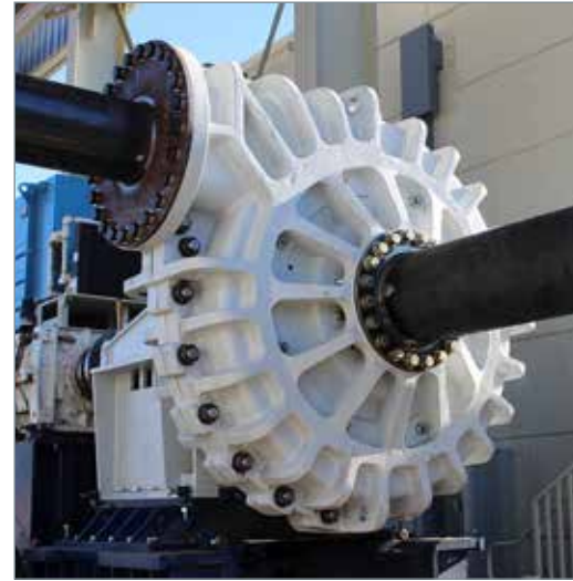
Krebs slurryMAX XHP extra high pressure pump.
