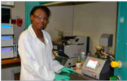
Senior laboratory technician at WearCheck, Lizzy Chabangu, operates the condition monitoring company's brand new PMA5 Pensky Martens closed cup flashpoint tester in Johannesburg recently.
