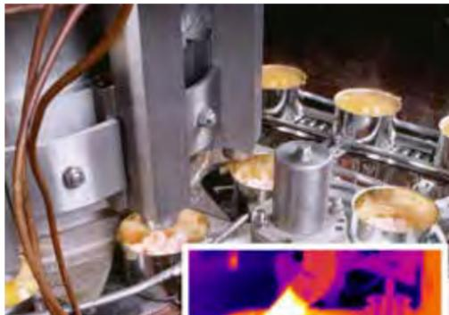
By comparing similar bearings, infrared easily spots where there is a problem. In this case, two bearings on these rollers are nearing failure, which could shut down this line.
