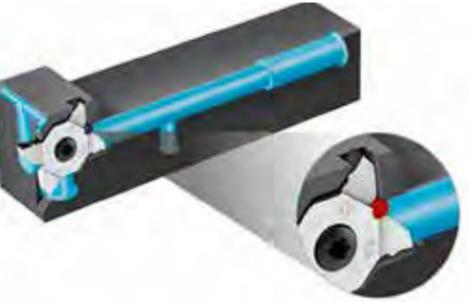
self-aligning tangential clamping, the insert is pressed against the contact points when the screw is tightened. A special dowel pin helps with accuracy of fit and simultaneously makes it impossible to mount the insert incorrectly. That results in a high degree of dimensional stability and repeat accuracy. The fact that the insert
