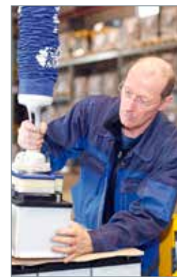
Vacuum tube lifter for starter batteries from Hytec.
