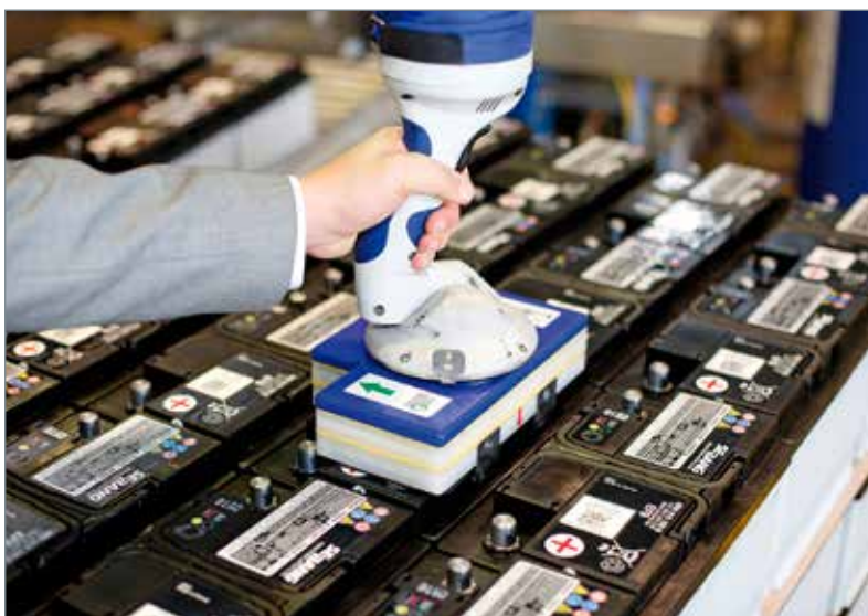
The Schmalz vacuum tube lifter JumboFlex Battery provides a complete solution for the ergonomic and safe handling of starter batteries.
