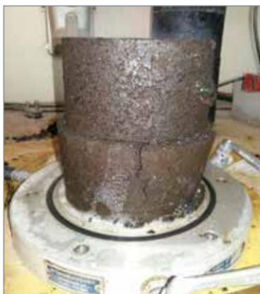
*Asphalt briquettes after mist conditioning to assess the performance of the different mixes in the Grey Water Study.*
