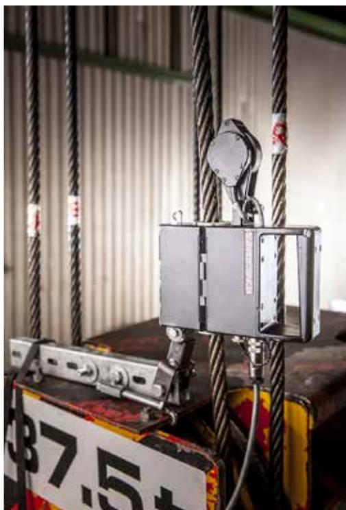
much faster, remotely operated robot combined with a visual inspection to provide you with an in-depth view of the alignment and condition of the crane rail. RailQ measurements include span, straightness, elevation and rail-to-rail elevation.
