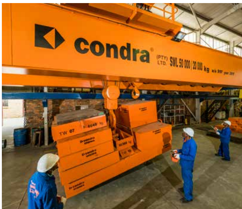
Exxaro's 18,4m span 50/20t machine featuring variable frequency drives on the main lift, long travel and cross travel to facilitate precise positioning of very heavy loads, under test in Condra's Johannesburg factory.
