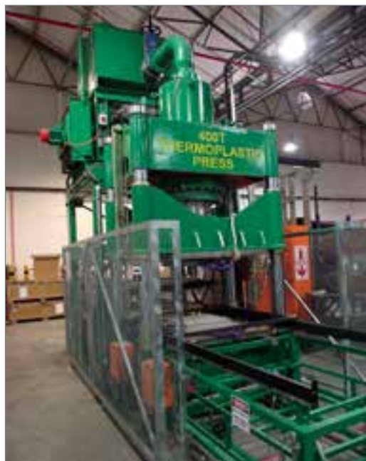
The Hytec-supplied 400-ton thermoplastic press, which is used in deep-moulding composite materials for components in the aerospace industry.
