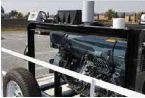
A simulation was done using an older model trailer mounted diesel engine supplied by ECS that was equipped with a Booyco PDS.
