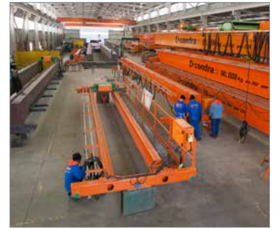
Typical overhead cranes under manufacture in Condra's factory.
