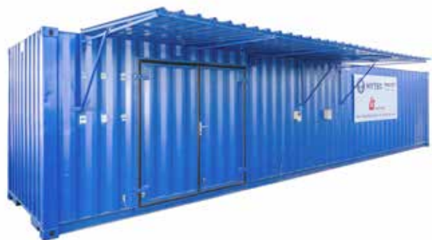
The bolt-on canopy is used to accommodate the hose cut-off machine, which is normally situated outside the container in order to adhere to most mines' health and safety regulations.
