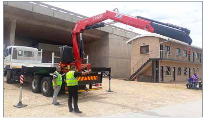
The crane truck has a lifting capacity of 10 tons and can serve as a giant fishing rod in port.
