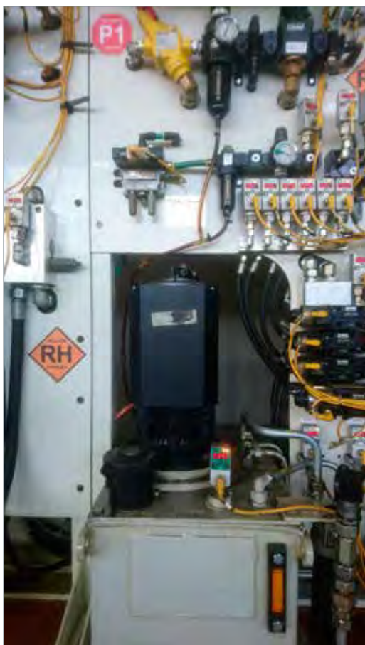
The Sytronix Variable Speed Pump Drive monitors the hydraulic pressure and adjusts the motor running speed so only the required pressure at any given time is delivered.
