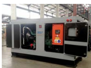
Diesel generator set housed in a sound attenuated container
