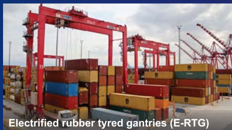
Electrified rubber tyred gantries (E-RTG)
