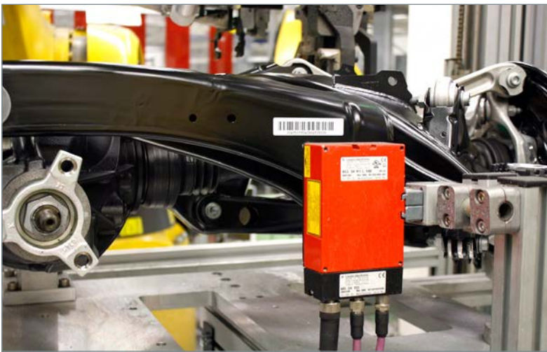
Engineered with a high tolerance to different materials, the Leuze 10 Series optical sensors are able to detect objects and measure distances with an incredible accuracy of +/-30mm.
