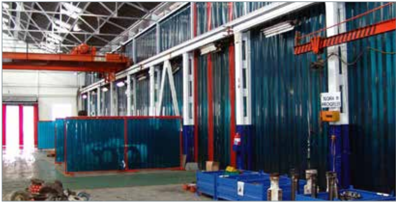
Apex Welding and Safety Screens are most often used to cordon off welding and grinding bays.
