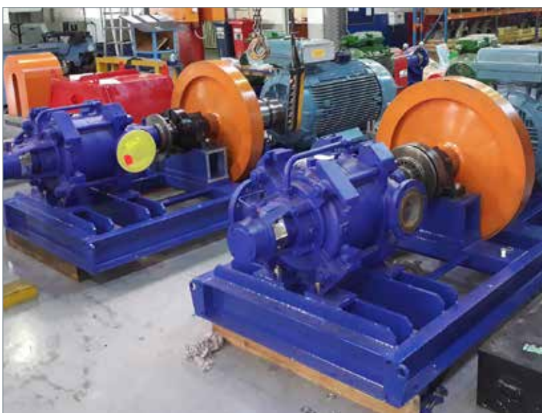
A unique flywheel water pump system that is able to continue pumping long enough to mitigate the possible effects of water hammer in the event of power failures was developed by KSB Pumps and Valves
