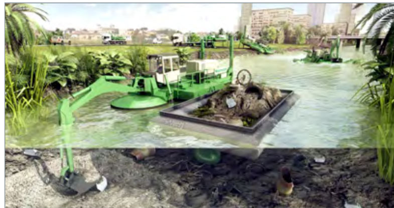
The mobile Webmaster is a specifically designed multipurpose dredger for shallow water environments.
