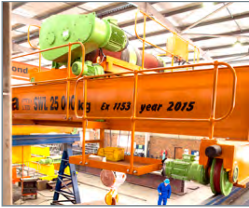
Load testing on one of the two 25 ton headgear cranes manufactured by Condra for Mopani Copper Mines' Sinclinorium shaft.
