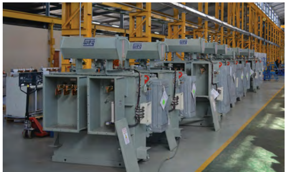
5 x 1 600 kVA 11 kV/433 V and 1 x 2 000 kVA 11 kV/720 V Transformers Export to Ghana
