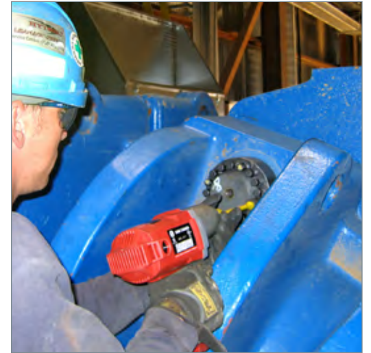
BMG's Superbolt multi-jackbolt tensioners, which form part of the Nord-Lock range, are designed to reduce downtime and eliminate unsafe and laborious bolting methods for pumps and pumping equipment, particularly in harsh operating conditions.
