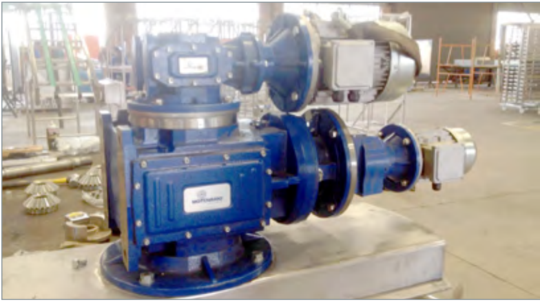
Motovario double reduction counter rotating auger drive.
