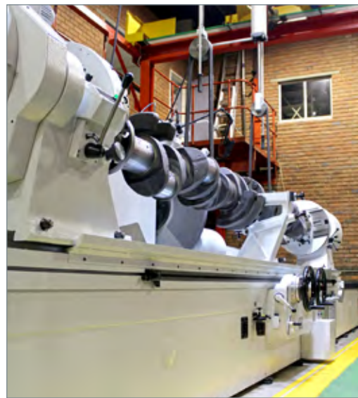
According to the company, the largest crankshaft grinding machine in Africa is hard at work at Metric Automotive Engineering.
