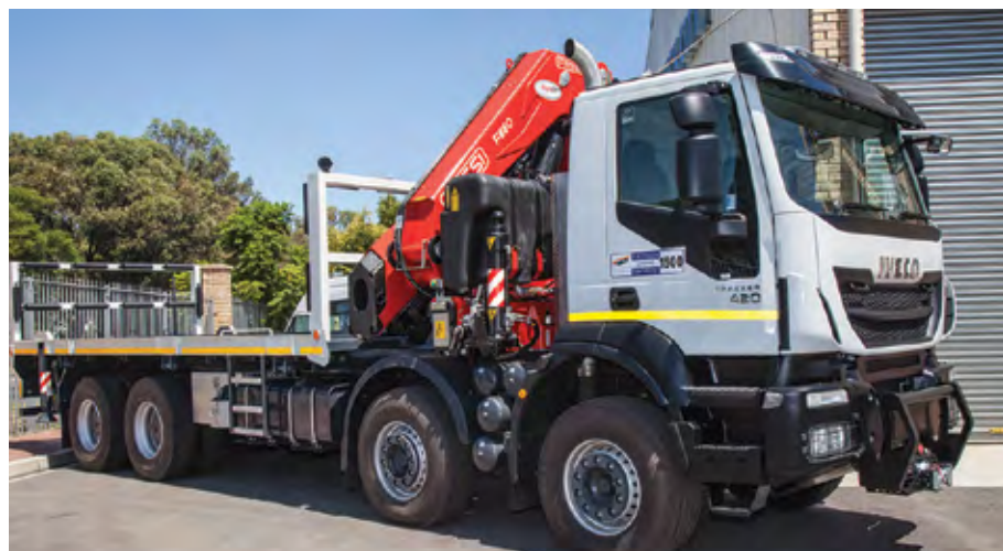
The first of three 9.5t capacity FASSI 660 RA 2.28 truck mounted cranes equipped with the latest FSC/SII stability control systems, mounted on IVECO trucks for the City of Cape Town Electrical Department.
