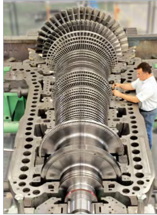
The 48MW TGM multi-extraction condensing steam turbine rotor, which is designed to maximise efficiency and power generation capability.
