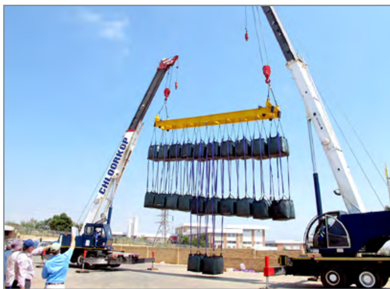
A load test being conducted on a beam designed and manufactured by Elephant Lifting Equipment for lifting multiple 1t sugar bags at a sugar-processing facility.
