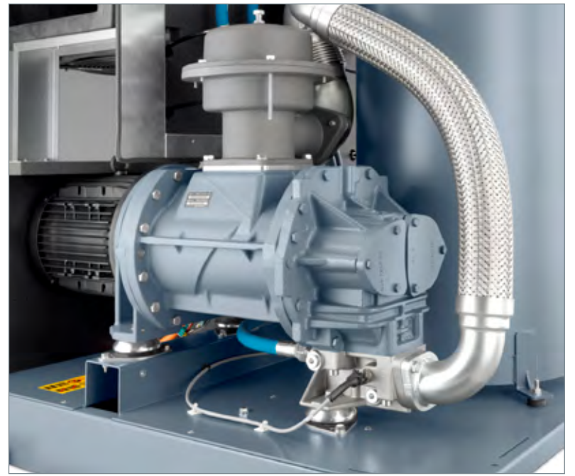
Combination of VSD technology of Atlas Copco rotary screw vacuum pumps and innovative new patent inlet valve provide modulating vacuum control to minimise energy consumption
