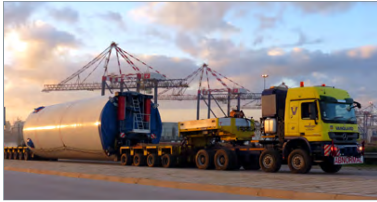
Abnormal transport: Vanguard transporting an 87 tonne Tower Section with Vanguard Tower Clamps on a Gooseneck 10 Axle Goldhofer THP-SL modular trailer combination for Metrowind’s Van Stadens wind farm.
