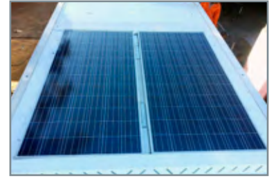
The solar panels eliminate ± two to four hours of idling per day for each trailer.
