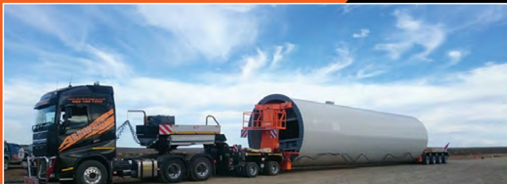
Wind tower adaptor trailer
