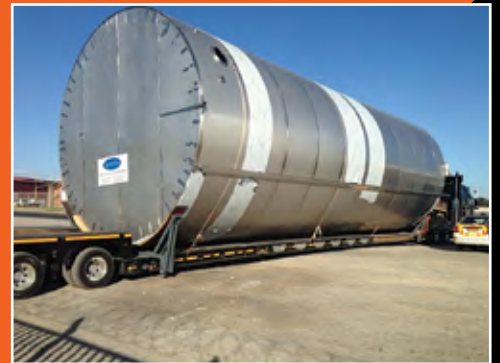
5,5m Diameter 18m long stainless steel tank
