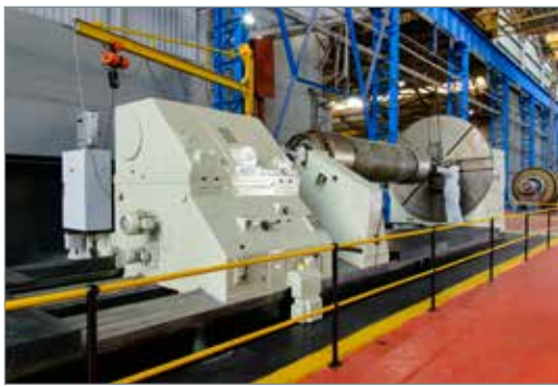
The newly installed 140 t lathe at Marthinusen & Coutts' power generation repair facility.
