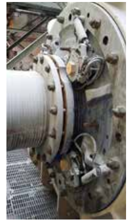
Adjustment mechanism reduces throatbush wear.
