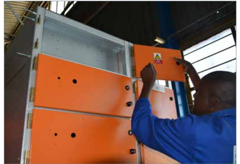
A live control voltage 110 Vac door being installed on a Shaw Controls aluzinc motor control centre.
