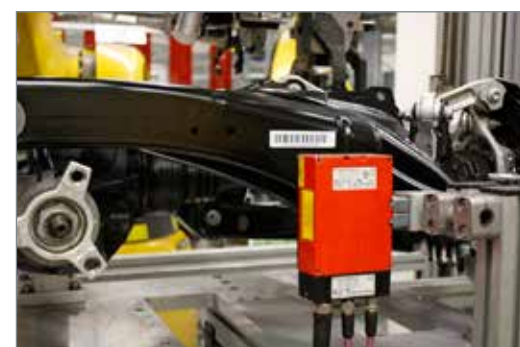
Engineered with a high tolerance to different materials, the Leuze 10 Series optical sensors are able to detect objects and measure distances with an accuracy of \pm 30 mm.
