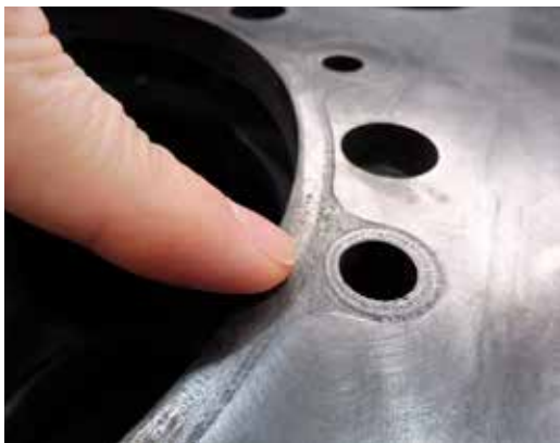
The worst degradation occurs at the block face where it meets the cylinder head.
