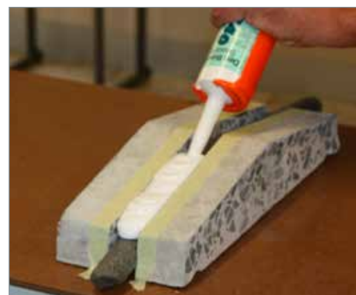
Den Braven Hybriflex-540 - applying with a polyethylene backing cord as a bond breaker.
