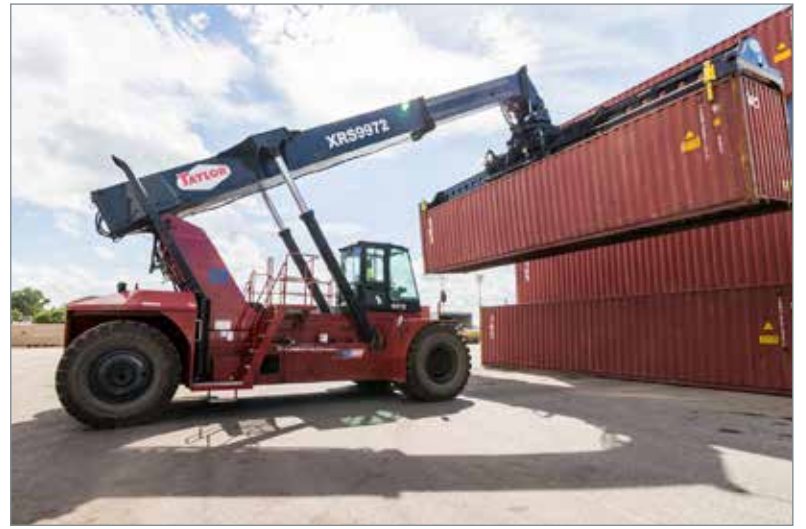
BLTWORLD's Taylor XRS-9972 reachstacker, with a high-strength telescopic boom, is designed to handle loaded containers stacked up to five high in the first row, four high in the second row and three high in the third row.
