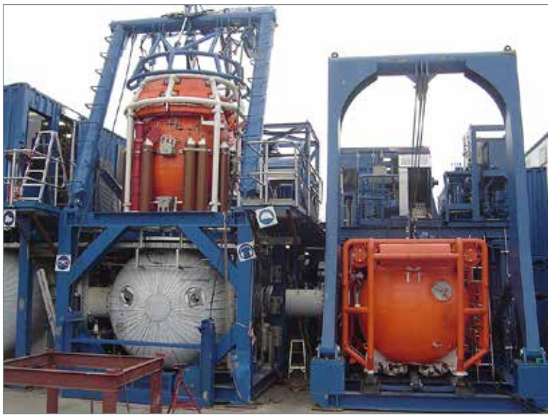
This diving system - designed and manufactured by Hyflo - is used in applications where divers are lowered to deep sea levels, when working on oil rig pipelines and oil wells. This is typically referred to as pressure-saturation diving.
