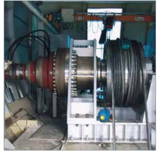
Typical application of Dinamic Oil gearbox, used to lift, turn and hold railway coaches securely in place during maintenance procedures, like welding and machining.
