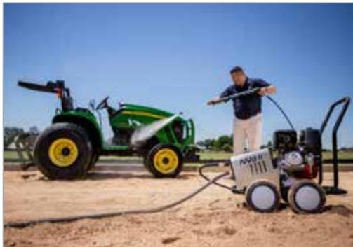
harvesters, crop sprayers and tractors clean. "High-pressure washers ensure that these big and expensive machines are maintained properly by removing any dirt particulates and general grime on a daily basis in wash bays, thus reducing maintenance costs and, of course, downtime," says Esterhuizen.
