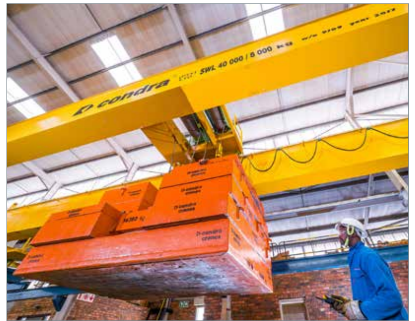
A typical Condra double-girder electric overhead travelling crane undergoing testing at the company's Johannesburg factory.
