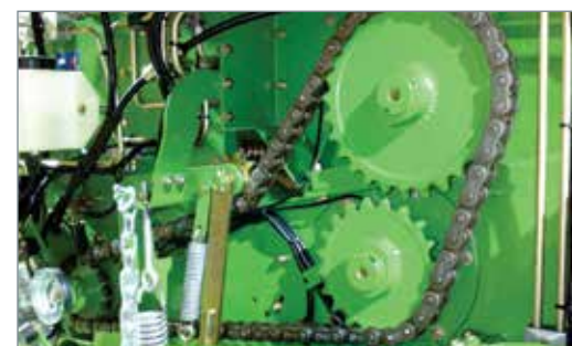
The robust Tsubaki RS100HT chain for balers has a 25% higher maximum tensile strength, improved anti-shock performance and greater fatigue strength, than competitive products.
