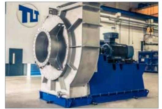
*The new TLT-Turbo fan for Mechanical Vapour Recompression.*
