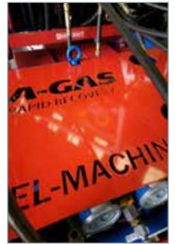
A-Gas Rapid Recovery machines are based on the simple concept of a compressor and a condenser.
