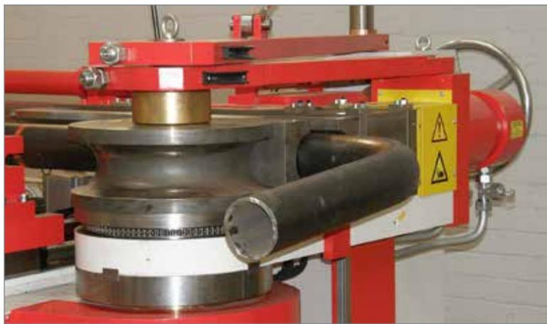
Demonstration bending of 100 mm mild steel pipe, accomplished in less than a minute!
