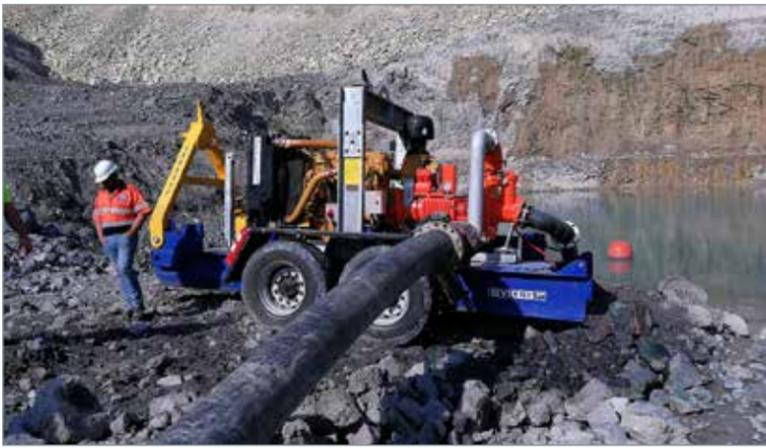
Equipped with automatic priming and solids handling capability, the Sykes Xtra High Head pump is ideal for harsh dewatering applications.
