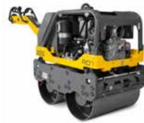
The Wacker Neuson portfolio of RD7 pedestrian rollers (RD7A, RD7H and RD7Ye) is ideally suited to applications that require the compaction of asphalt and granular material. These reliable, high-performance machines boast a smart and compact design that delivers a host of benefits. The tapered frame enables seamless compaction right up against walls or other boundaries and short roller spacing and low centre of gravity facilitates manoeuvrability.
