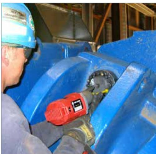
Although the primary benefit of Superbolt is the reduction of torque required, this device also reduces downtime and eliminates unsafe and laborious bolting methods, particularly in harsh operating conditions.
