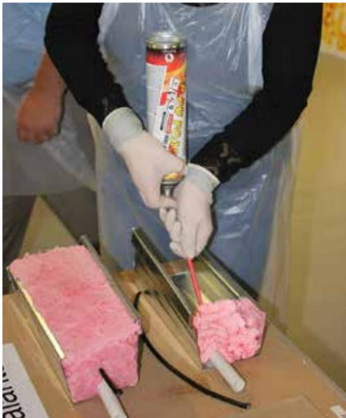
*Fire Protect PU Foam used to seal ducts and cable trays.*
