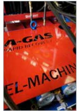
A-Gas Rapid Recovery machines are based on the simple concept of a compressor and a condenser.
