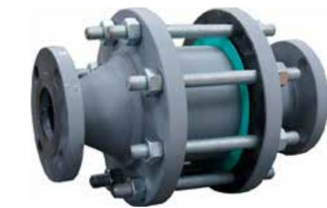
Flame arresters act as heat sinks by partitioning the flame into tiny flamelets and quenching the tiny flames.
