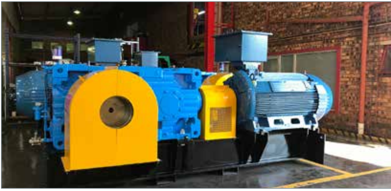
One of the nine-drive package units supplied to a greenfield copper mine in the DRC.
