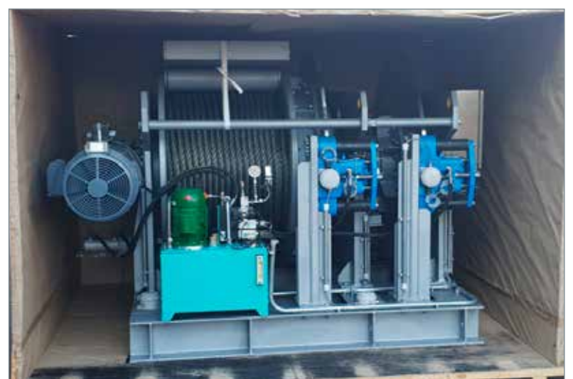
Dymot winch incorporating its disc brake system.
