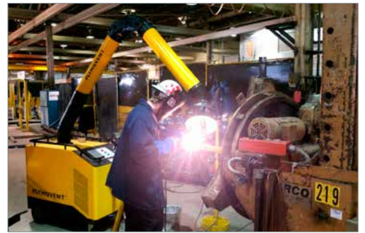
Auto darkening welding helmets, with integrated lightweight Powered Air Purifying Respiratory (PAPR) units, provide protection against eye and face injury, as well as preventing respiratory problems.
