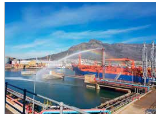
Testing the remote water cannon for fire protection in the Cape Town docks.
