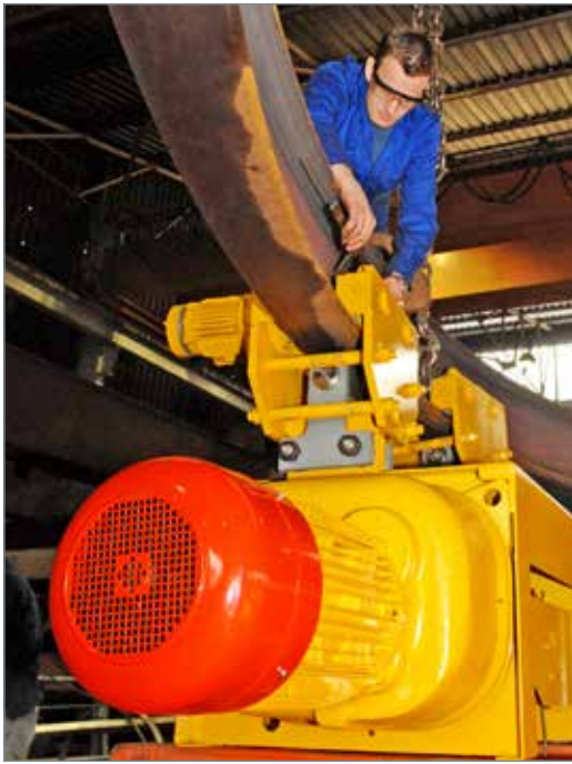
Typical Condra K-Series articulated hoist under test.
