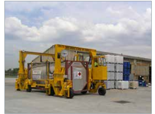
The Mobicon mobile container handling system ensures the safe handling, transportation and storage of hazardous and non-hazardous substances.
