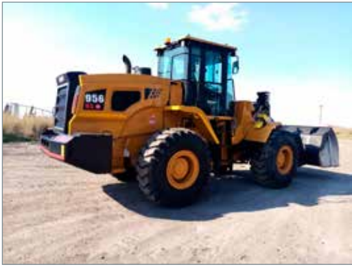
The SANY SYL956s were specially modified for this application with 4.6 cubic metre coal buckets.
