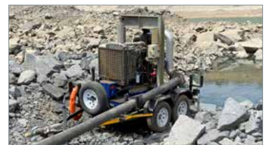
The Sykes CP units weigh only about 1,5 t on a road trailer, which allows easy mobility on-road and off-road.
