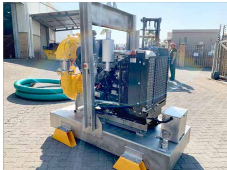
A custom engineered stainless steel Sykes pump set produced by Integrate Pump Rental.
