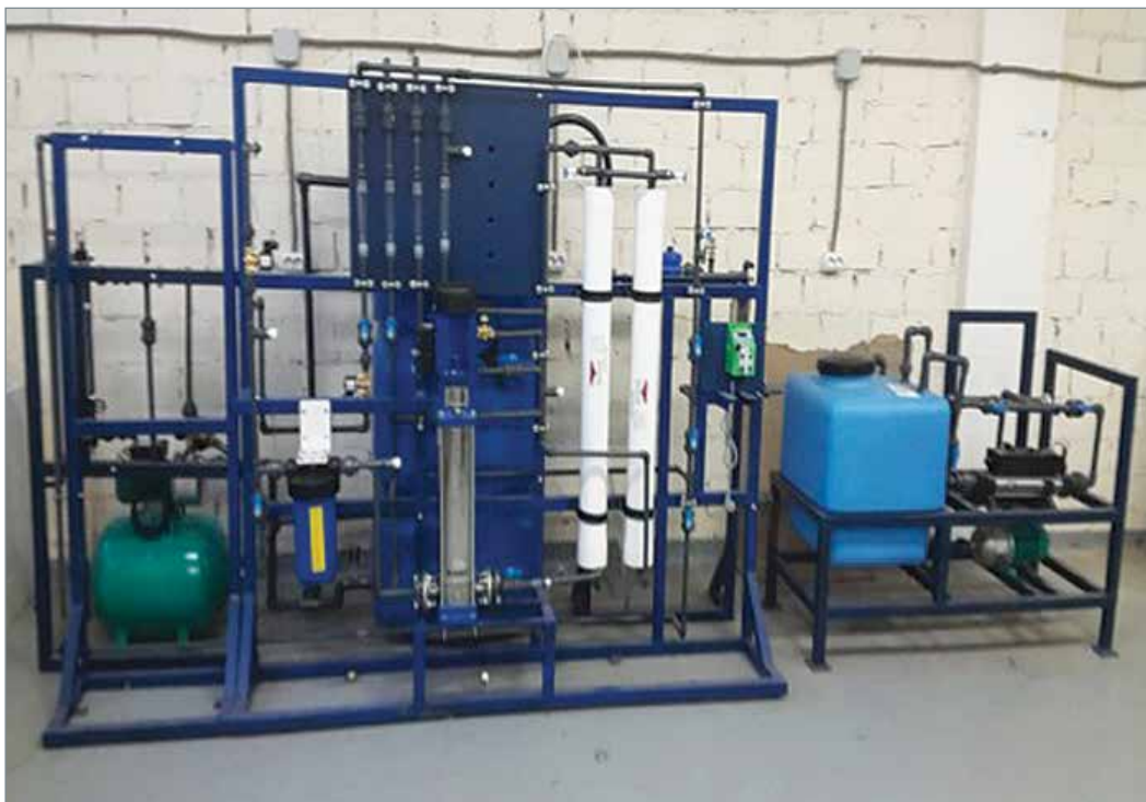
Rosatam Rosa-TM-15 water treatment unit.
