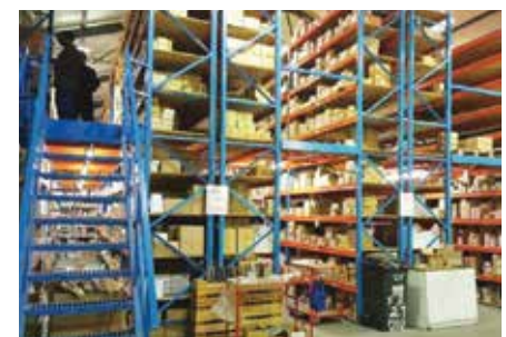
Rack supported multi pick levels
