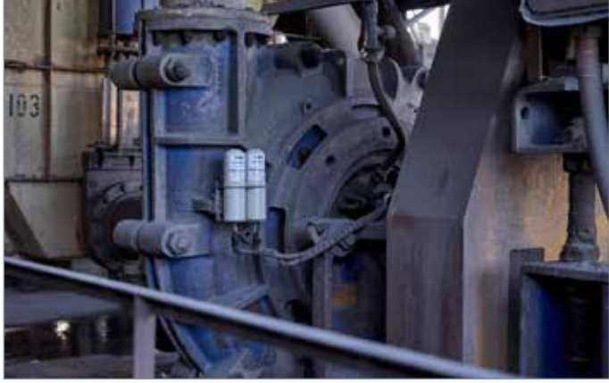
Accumin lubricators ensure optimal performance for Warman slurry pumps.
