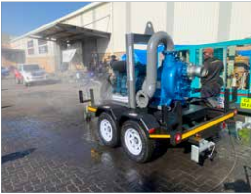
Trash pumps can typically handle solids up to 76 mm in size with flow rates of up to 110 l/s at maximum head of 32 m.
