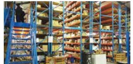
Rack supported multi pick levels
