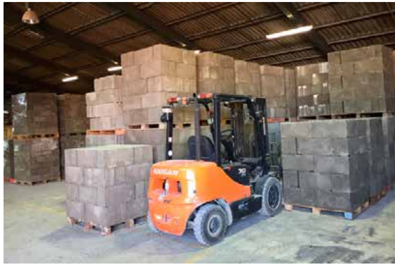
Lightweight concrete bricks made from recycled polystyrene.
