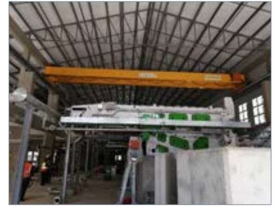
The Condra 4-ton, 14,7-metre span double-girder electric overhead travelling crane already installed at Zandvliet Wastewater Treatment Works.
