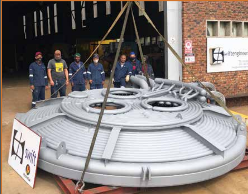
SwiftNova Engineering recently manufactured and delivered an arc furnace roof to PetroSA's GTL refinery in Mossel Bay. This intricate part of the GTL process is a first of its kind to be built by a local company.
