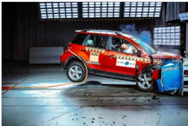
Renault's Kwid under performing in offset crash test.
