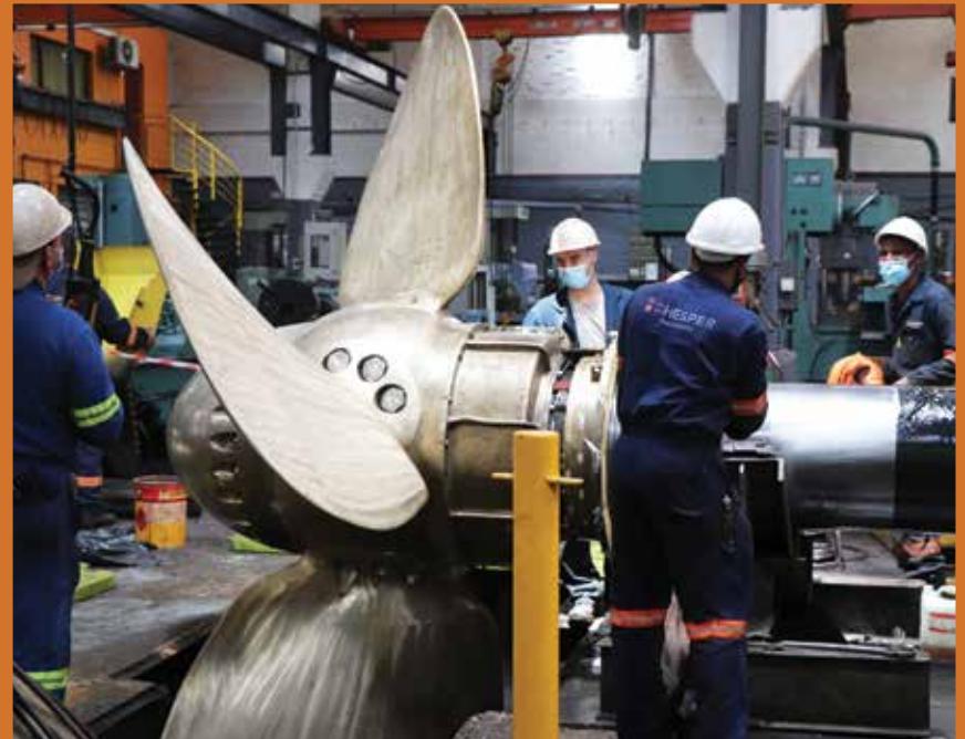
Hesper Engineering is known for being the propulsion specialists in the marine industry. The 25 ton, 400mm OD tailshaft pictured was removed from a fishing vessel, the Trondheim and was inspected, repaired and fitted back in a quick turnaround time.
