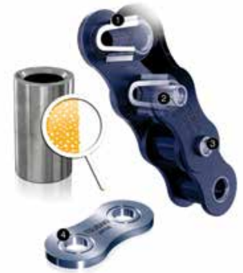
Tsubaki Lambda lubrication-free chain – four key features: 1. Sintered oil-impregnated bush, 2. Specially coated pins, 3. Centre sink rivets and 4. Ring coin.
