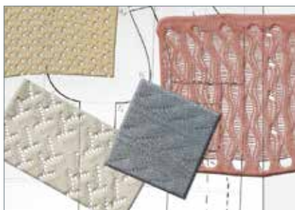
MIT engineers have developed self-cooling fabrics from polyethylene, commonly used in plastic bags. They estimate that the new fabric may be more sustainable than cotton and other common textiles. Credit: Svetlana Boriskina
