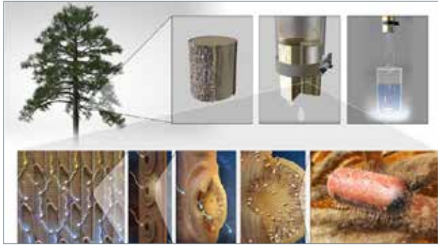
Xylem tissue in gymnosperm sapwood can be used for water filtration (as seen on top). Xylem is comprised of conduits that are interconnected by membranes that filter out contaminants present in water (bottom). Credit: N.R. Fuller, Sayo Studio.
