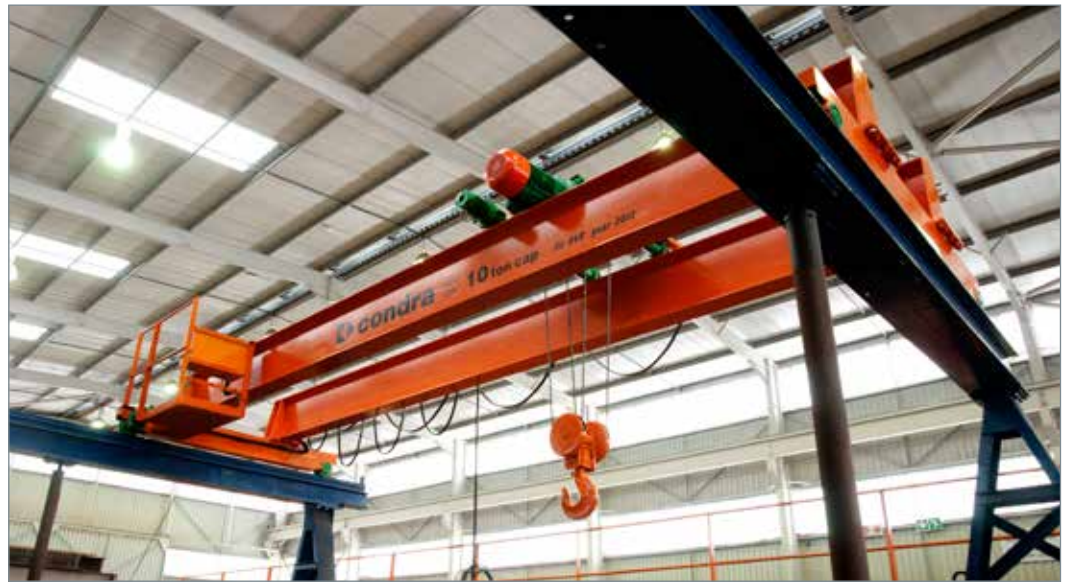
Typical Condra double-girder electric overhead travelling crane, similar in arrangement to the seagoing crane, but with the motor drive delivered to steel wheels instead of rack-and-pinion.
