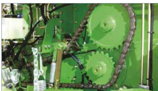
BMG’s Tsubaki RS100HT chain for balers has a 25% higher maximum tensile strength, improved anti-shock performance and greater fatigue strength, when compared to other chain.
