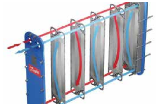
The flow pattern in a gasketed plate heat exchanger.
