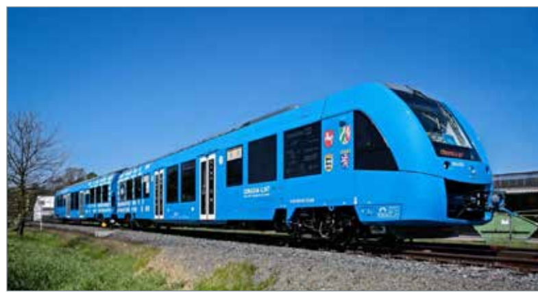
Alstom's Coradia iLint, the world's first hydrogen powered train.
