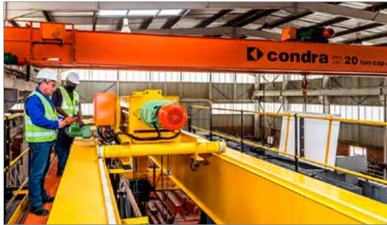
A Condra overhead crane (yellow), similar in overall design to the cranes being manufactured for the new vehicle plant, seen here under test in the Johannesburg factory.
