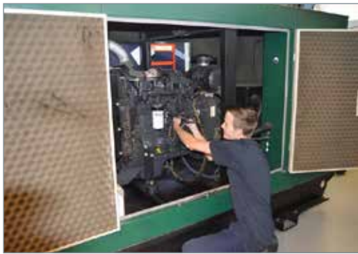
Specialist repairs on a generator diesel injection system underway at Reef Fuel Injection Services.
