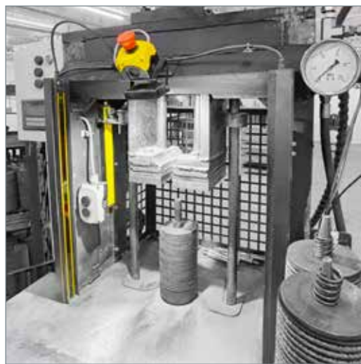
Following successful installation of ReeR light curtains IWT Abrasives has realised an improvement in operator efficiency by almost 20%.
