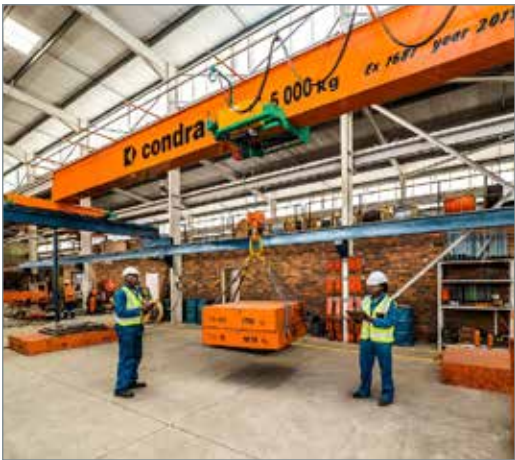
A Condra 5-ton single-girder overhead crane.
