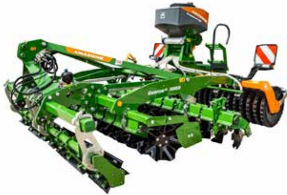
The X-Cutter disc is available as an option for new orders or for retrofitting to various models from the Catros+ and CatrosXL compact disc harrow range.
