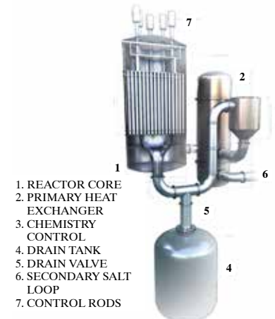
Infographic of Seaborg Compact Molten Salt Reactor. Reactor vessel's height is 2.4m and the diameter is 2.2m. Thermal capacity: 250 MWt, Electrical capacity: 100 MWe.
