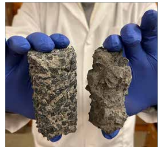
Comparison of a concrete sample coated with nano-modified sealer (left) versus untreated concrete (right). Credit: WSU.
