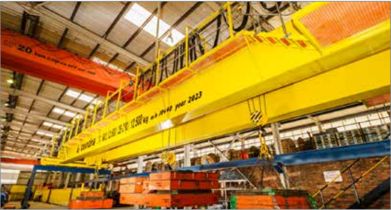
Saiccor Mill's 12,5/25/12,5-ton overhead travelling crane under factory load test before delivery.
