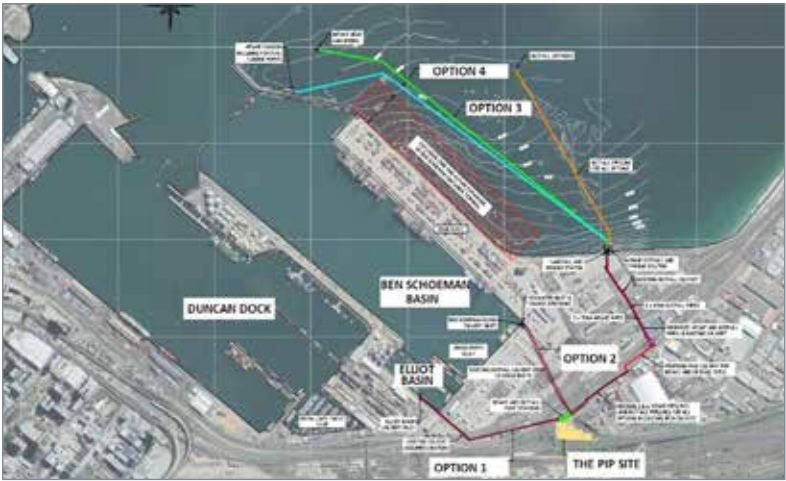
Intake options investigated for proposed desalination site.
