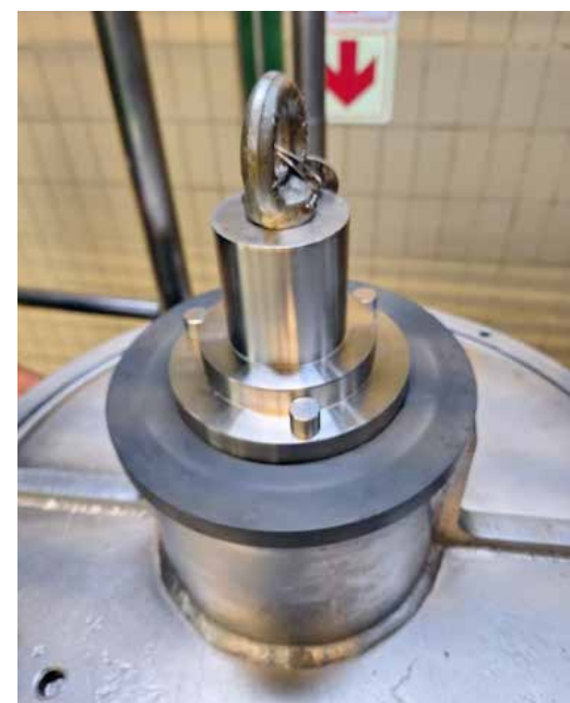
A Vesconite thrust washer has been successfully employed on a grinding machine at a large fruit juice concentrate producer.
