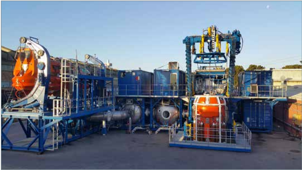
A DNV classed 12-man customised saturation diving system manufactured in South Africa by Unique Group
