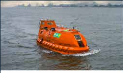
Self-Propelled Hyperbaric Lifeboats
