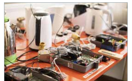
Smart geyser prototype testing station - kettles are used to test the devices
